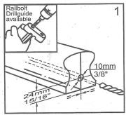
Mark position of 10mm 3/8" hole onto end of rail. As an alternative to marking hand rails for drilling, the Railbolt Drill Guide is available making it fast and easy.
