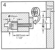
Assemble the shaft and gear housing into the rail.
