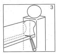
Mark fully final position of the handrail onto post observing the centre line.
