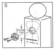
To mark the centre of the keyhole disc measure 28mm 1 1/8" upwards from the bottom of the rail position. Using a 25mm 1" bit bore hole into post 7mm 9/32" deep so the keyhole disc is flush or slightly under. Secure disc with screws
