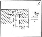
Mark and bore 25mm 1" and 10mm 3/8" holes as indicated.
