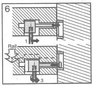
The shaft should be flush or under the surface of the rail end. Using a 5mm hex bit in a tool or Allen wrench fitted into the gear housing the shaft can be moved to engage into the disc keyhole. Then simple push rail downwards and tighten.
