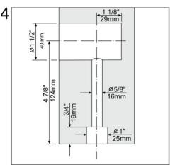
**4.** Mark the center point of the 1 1/2"-38mm hole on side of the post and bore to recommended depth. Mark the center of the post base and bore the 1"-25mm hole 3/4"-19mm deep. Now using a 5/8"-16mm continue boring through the centre of the 1"-25mm hole until reaching the 1 1/2"-38mm hole. Ream the 5/8"-16mm hole if necessary. The 1"- 25mm hole allows the post to sit freely over the hex nut on the Base Plate.
