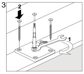
3. Slide the Base Plate over the shaft. Tighten clockwise until it reaches the decking with 17 mm wrench to desired position. Install the 4 screws. (For maximum strength, ALL SCREWS SHOULD BE INSTALLED)
