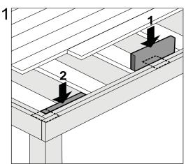
1. Add additional blocking as needed to accept all four screws and center lag screw.
