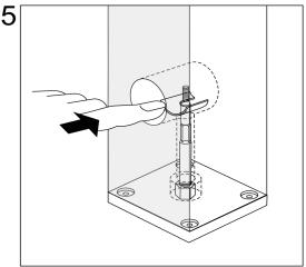
**5.** Position post over screw shaft and slide the curved washer making sure it is pushed to the to the very end around the screw shaft.
