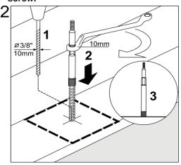
2. Bore the center pilot hole 3/8"-10mm. Tighten lag end into the wood with 10mm wrench stopping at the point of the machine thread that will receive the Base Plate. If needed, use some wax for lubrication on the lag portion of shaft to ease installation.
