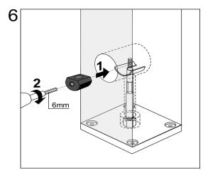
**6.** Finally install the gear housing onto the screw shaft, tighten using a 6mm hex bit (provided) in a power or hand tool. Finish off with a wood plug (not included) as needed or slide post cover over wood post at this point.
